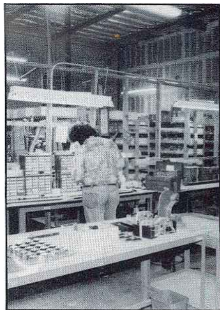
Adjacent to the electronic assembly area is a mechanical assembly section, where mechanical components are fitted together and circuit boards are installed in larger systems.
